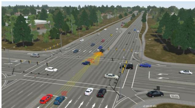
VTD helps to develop the complex environments with complex traffic modules and intersections with more than 200+ participants in it. Also, the pedestrians with interaction with the environment can be added to the scenarios.
