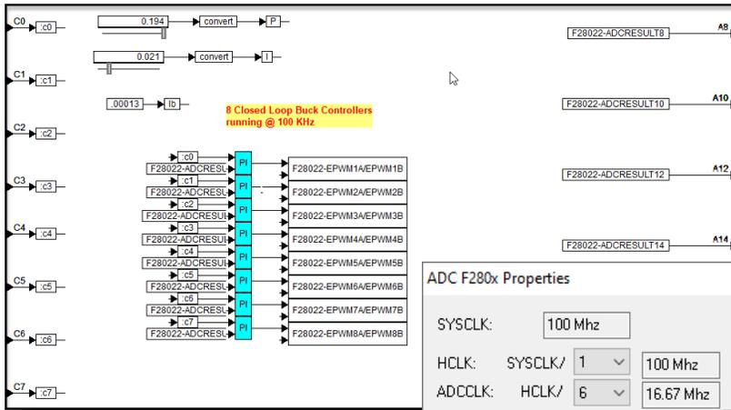
Embed model of a 400 kHz digital buck voltage converter that uses a built-in optimizer to tune the PI control against the simulated buck circuit (left). Once the controller gains are tuned, the embedded control is created with ADC input synchronized to the PWM output, along with background tasks to monitor temperature and set status LED bank (below, left). Embed auto-code generation creates the C file used to implement the control on the target (below).
