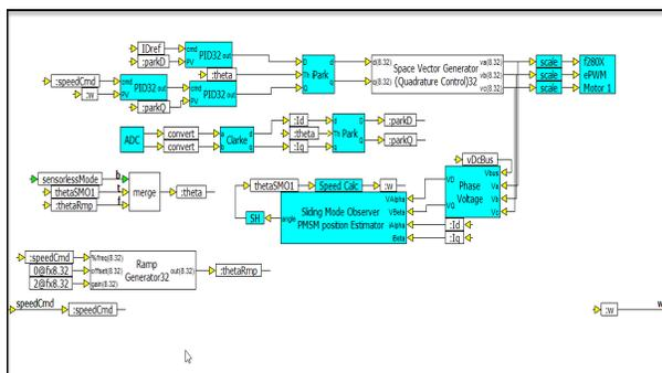
Subsystem 1 of two sensorless PMSM motors using sliding mode observer estimation of rotor position. Sample rate is 10 kHz running both motors on a Piccolo F28036 with 50% utilization.
