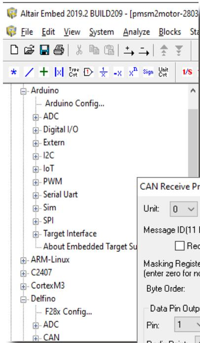
Use the collapsible Block Browser in the left windowpane to drag target-specific blocks to a diagram.
