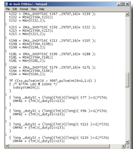
generated execution file. For example, code generated for closed-loop motor control—including, PI controller, digital output, PWM, and encoder peripherals—runs at 300KHz on a 150MHz F28335 DSC. The memory footprint is:
