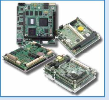
Conduction **Cooled SBCs** Higher reliability and wider operating temperature ranges
