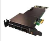
Relyum has launched an innovative edge computing product for the Smart Grids, aligned with the current virtualization trends. This device incorporates to the RELY-PCIe model a powerful processing capability for protecting and measuring the quality of the Electric grid based on the SV provided by the merging units.
